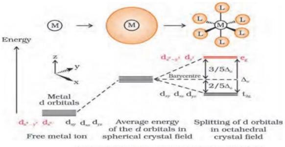
d orbital splitting in an octahedral crystal field
