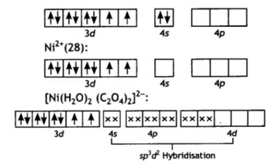
The complex has two unpaired electrons, therefore, it will be paramagnetic.
